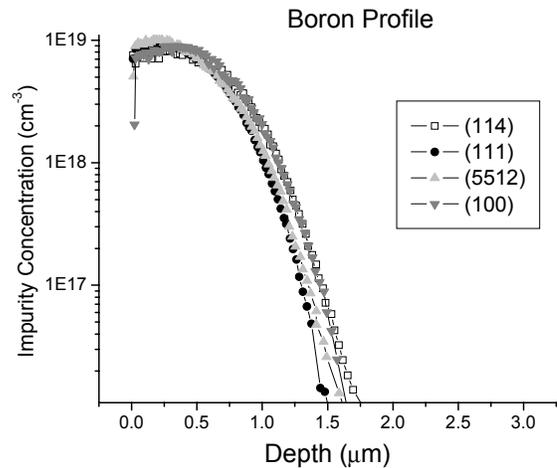
Fig. 1. Boron profile in Silicon as a function of the crystal orientation.
