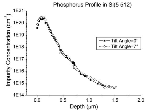
Fig. 2. Phosphorus profile in Si(5512) for two different beam angles (Similar results were found for Si(114)).
